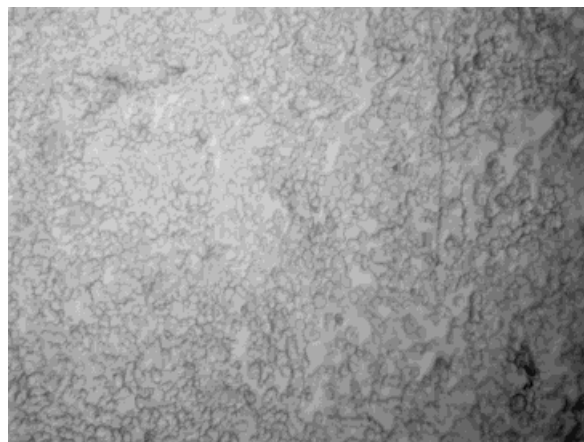
Figure 1 Photograph of the silica-filled rubber vulcanizate for the compound S1 obtained using an optical microscope ( \times 1000 ).
