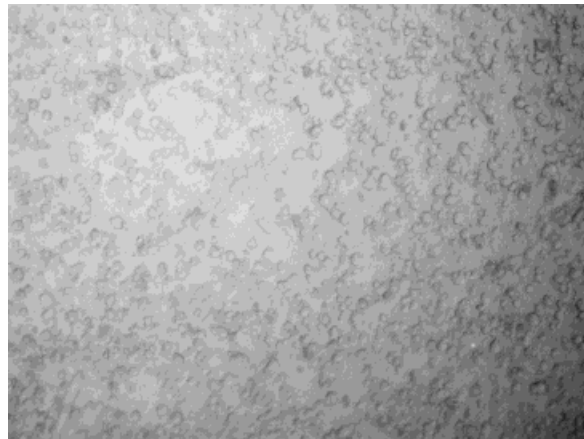
Figure 4 Photograph of the silica-filled rubber vulcanizate for the compound S4 obtained using a optical microscope ( \times 1000 ).
